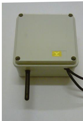
Box with lid attached, antenna must face ground & holes in box must be sealed.
