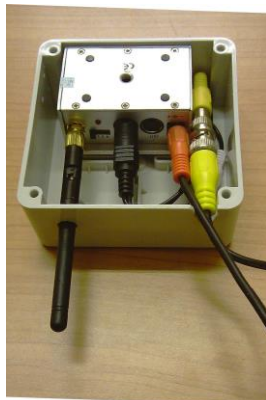
200 Meter transmitter in Outdoor waterproof box
